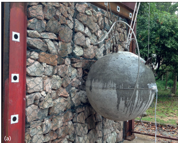
Figure 12. (a) Large-scale physical impact test on a rigid barrier with a gabion cushioning layer, and (b) centrifuge test to examine debris dynamic impact loading on a simulated flexible barrier
